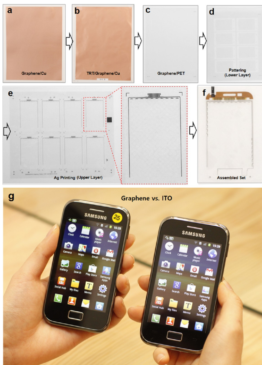
Figure 5. Photographs of the fabrication processes of graphene-based capacitive touch-screen devices. (a) Graphene on a Cu foil after RT-CVD growth. (b) TRT layer laminated on top of the graphene/Cu film at room temperature. (c) Graphene on a PET film after etching Cu and detaching TRT by hot laminating. (d) Patterned graphene/PET film by photolithography and O_2 plasma etching. (e) Screen-printed Ag electrodes on top of the patterned graphene electrodes. (f) Complete set of assembled layers including upper and lower graphene electrodes with an OCA layer in between. (g) Photograph of the graphene touch screen installed in a mobile phone (left) in comparison with an ITO-based touch screen phone (right).
